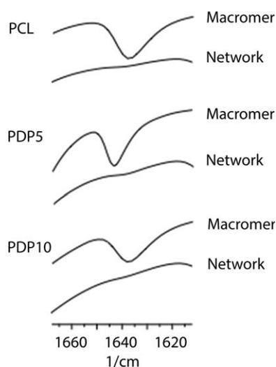
**FIGURE 4** FTIR transmittance curves attributed to the methacrylate double bonds before photocrosslinking (Macromer) and after photocrosslinking (Network).
