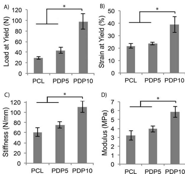
**FIGURE 9** (A) Maximum load at the yield point, (B) strain at the yield point, (C) stiffness, and (D) compression modulus of the scaffolds prepared by stereolithography.
