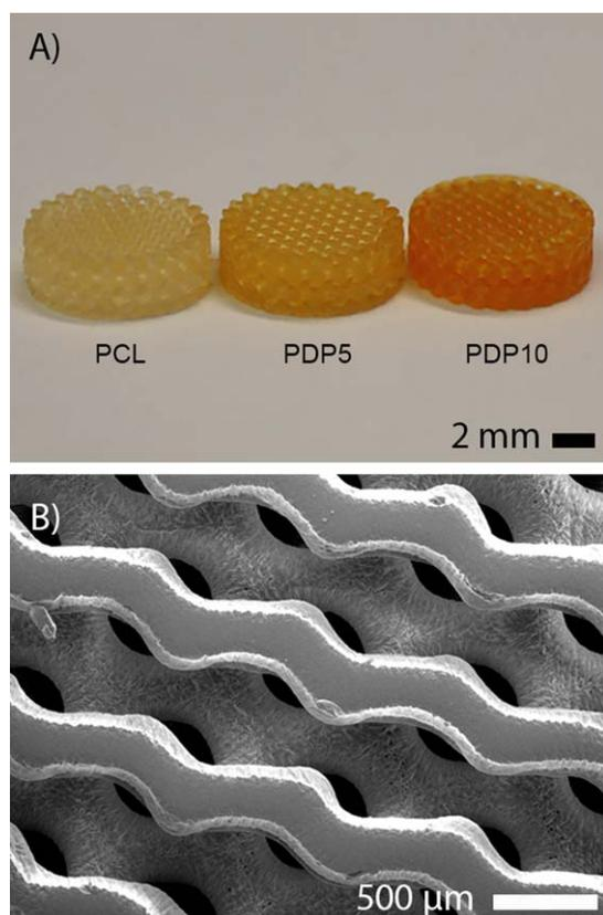
**FIGURE 8** (A) Photograph of the scaffolds prepared by stereolithography and (B) SEM image of the top surface of the PDP10 scaffold.
