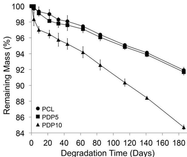
**FIGURE 5** Mass loss of the photocrosslinked polymers in PBS.
