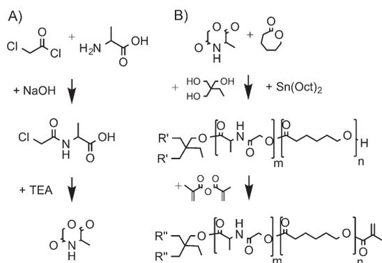
**SCHEME 1** (A) The synthesis of the cyclic MMD monomer and (B) the ROP of the cyclic monomers followed by the methacrylation of the star-shaped hydroxyl-ended oligomers.
