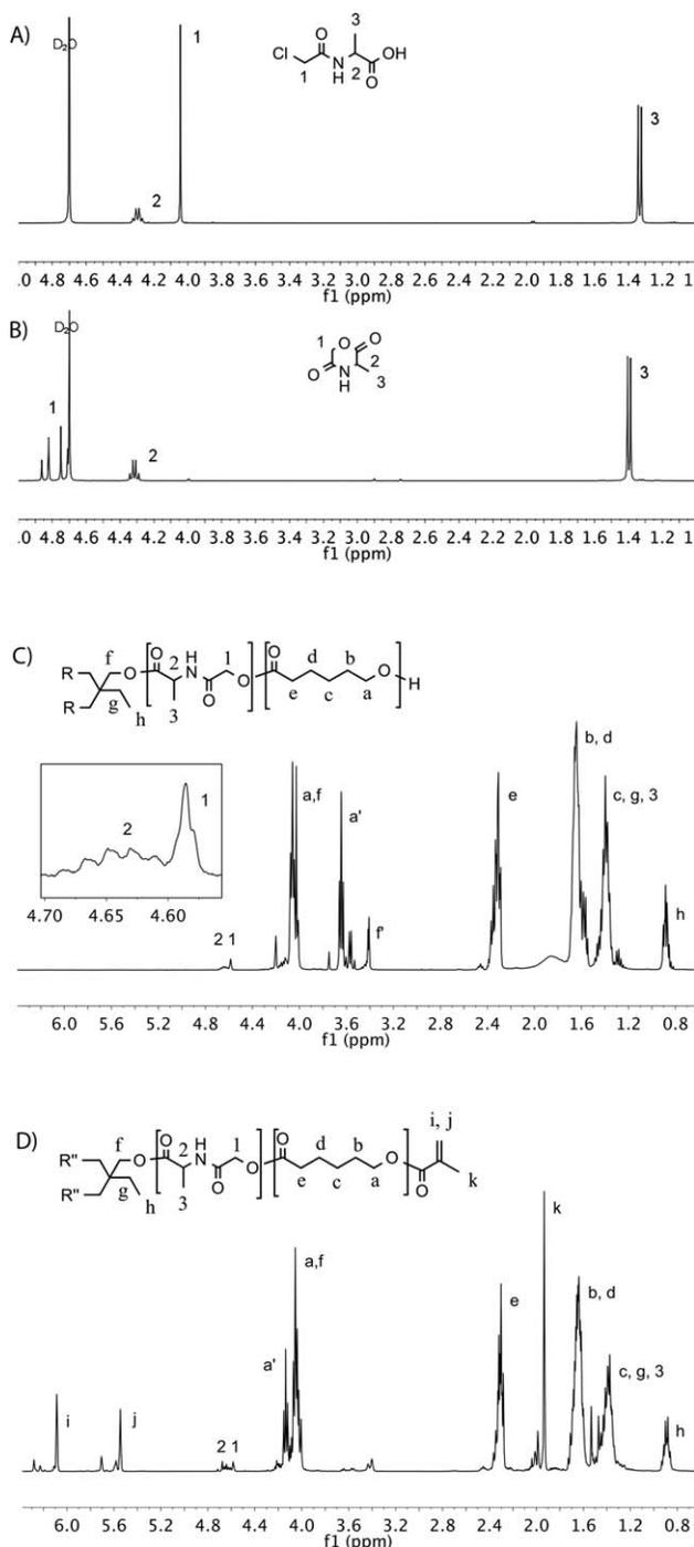
**FIGURE 1**  $^1\text{H}$  NMR spectrum of (A) *N*-chloroacetyl-L-alanine in  $\text{D}_2\text{O}$ , (B) MMD in  $\text{D}_2\text{O}$ , (C) PDP5 oligomer in  $\text{CDCl}_3$ , and (D) methacrylated PDP5 macromer in  $\text{CDCl}_3$ .
