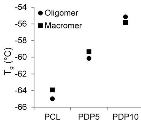
**FIGURE 3** Glass transition temperatures of the oligomers and the methacrylated macromers.
