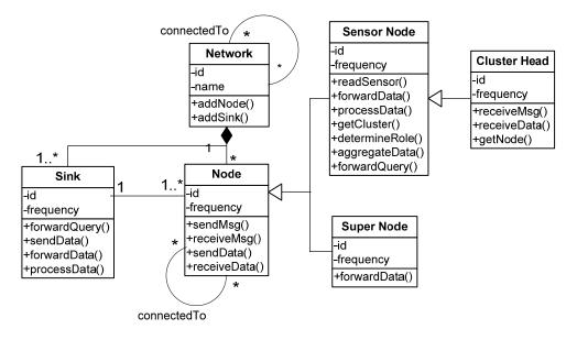
Figure 2. Class Diagram of a Wireless Sensor Network
