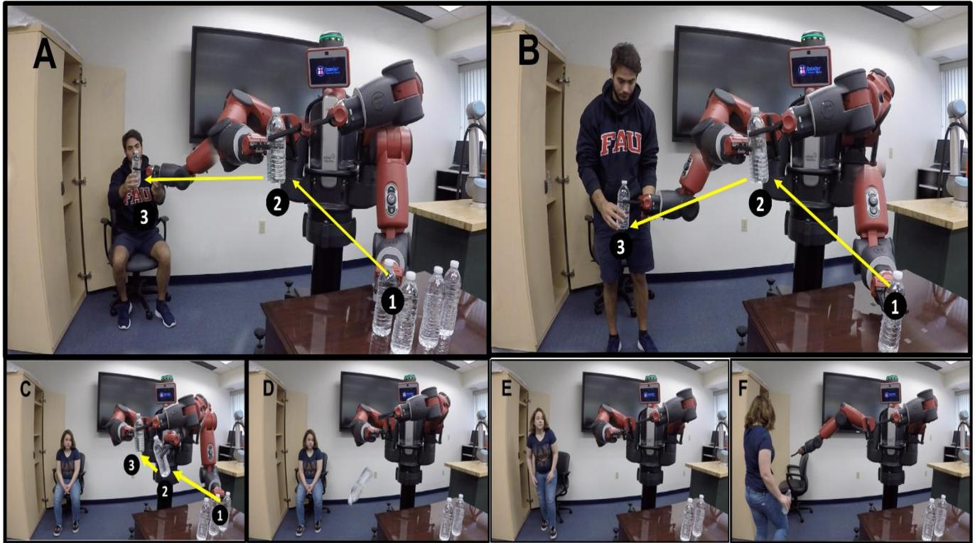
**Figure 2. Photo sequence of the Baxter Robot operation modes, (A). Successful placement, (B). Bottle Delivered to Wrong Location, (C, D, E, and F). Bottle Dropped**
