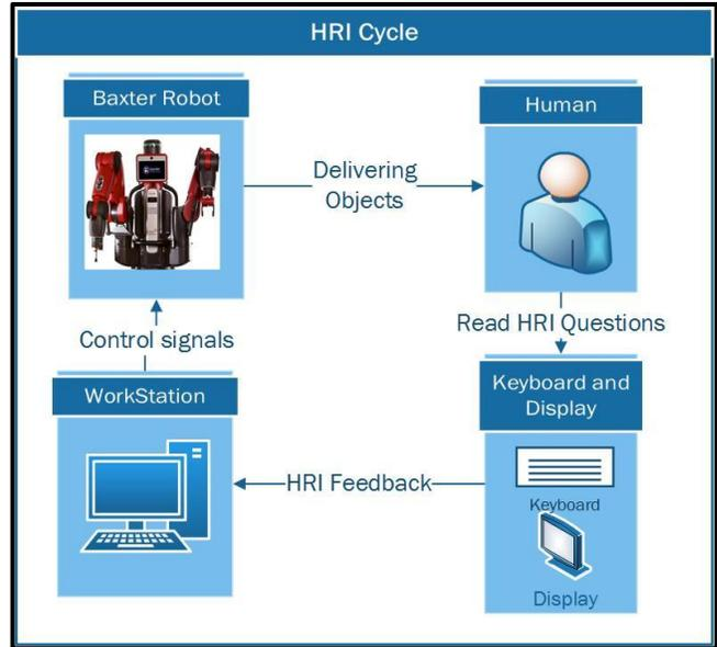
Figure 1. HRI Experiment Setup
