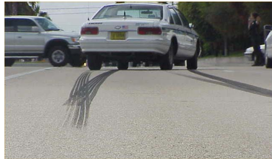
Figure 1. Typical locked-wheel skid marks.
