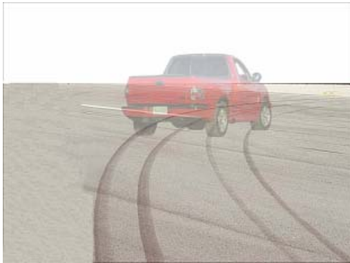
Figure 3. Tire marks from a vehicle side-slipping (yawing) while translating.
