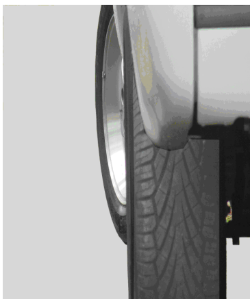
Figure 9: Front and rear tires are not parallel during steer maneuver (view from rear).
