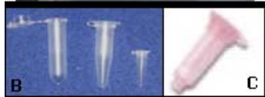
Figure 5. Equipment used for preparation of RNA from tissue culture cells: A) centrifuge, B) collecting tubes, and C) RNeasy spin column [14]
