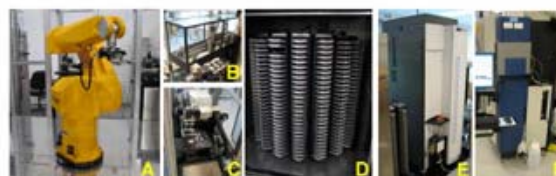
Figure 3. The Scripps Research uHTS platform. a) industrial anthropomorphic robotic arm, b) pin tool, c) liquid handlers, d) incubators, e) multimode plate reader, and f) kinetic imaging plate reader [6].
