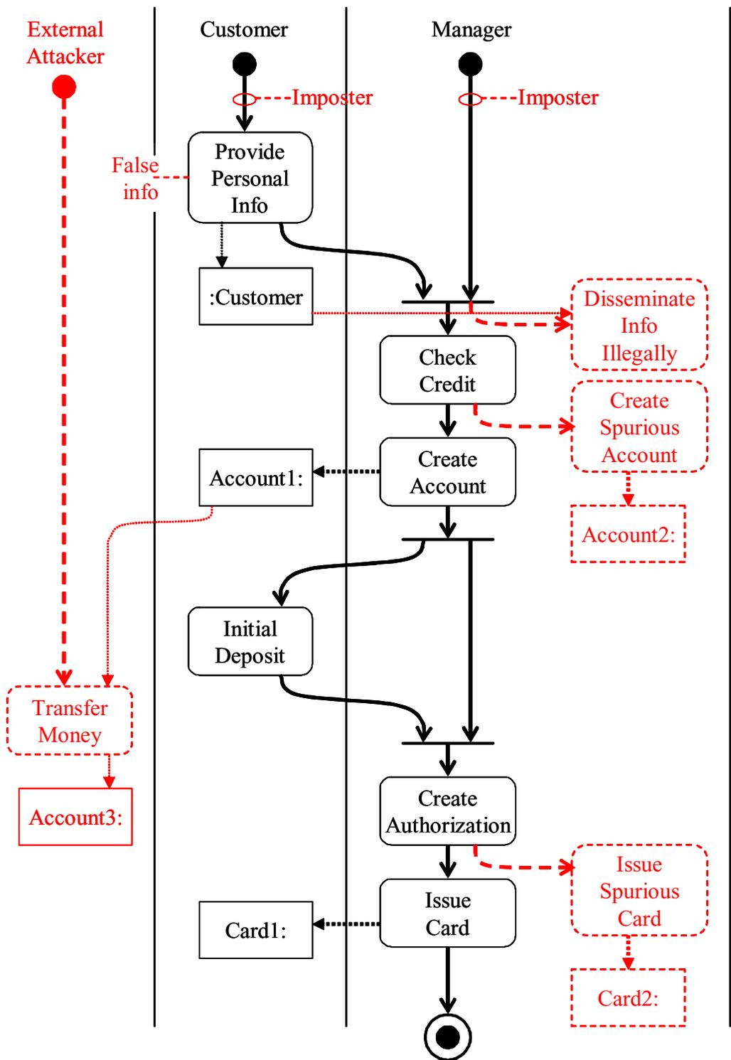
Figure 2. Activity diagram for use case "Open account".
