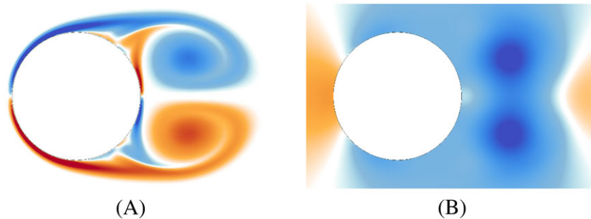
FIGURE 1 A, The vorticity field and B, the pressure field generated by flow over a stationary cylinder at Re = 1000 . Red regions correspond to positive vorticity and pressure, and blue regions correspond to negative values
