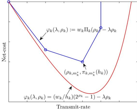
Fig. 2. Piecewise linear net-cost.
