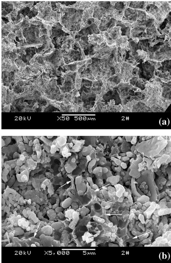
Fig. 2. SEM images of pore of composites scaffolds: section morphology (a) and the high magnification of inner pore (b). The white arrow on the photograph represents PLLA.
