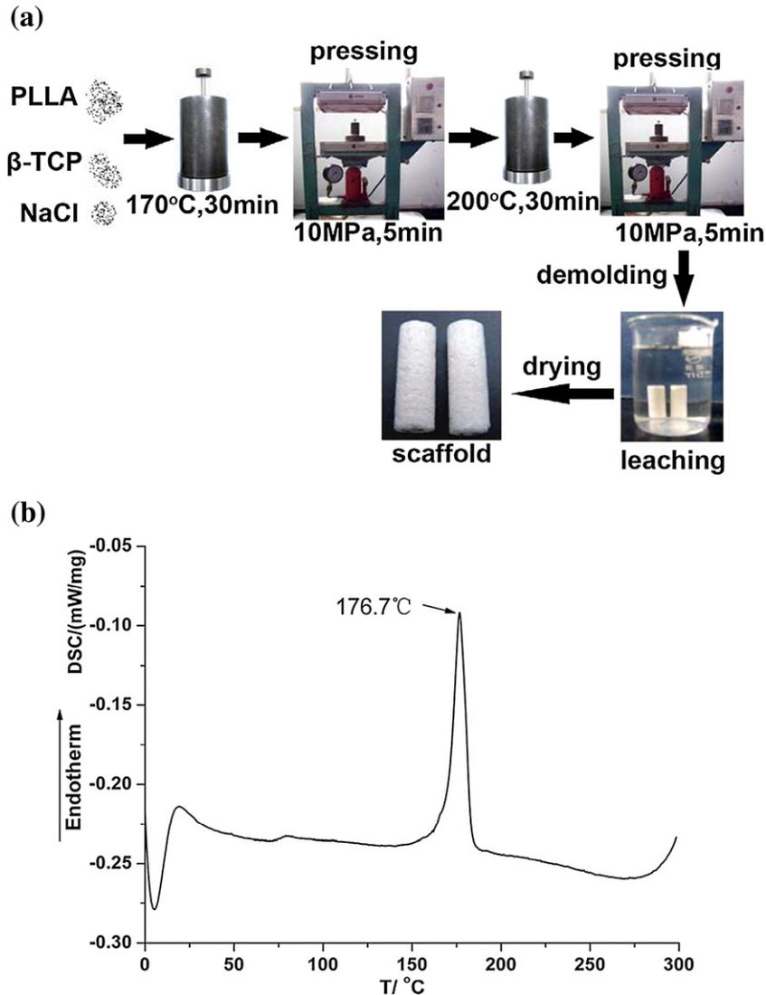
Fig. 1. Schematic graph of the whole procedure of novel PCLP method (a) and the DSC curve of PLLA (b).
