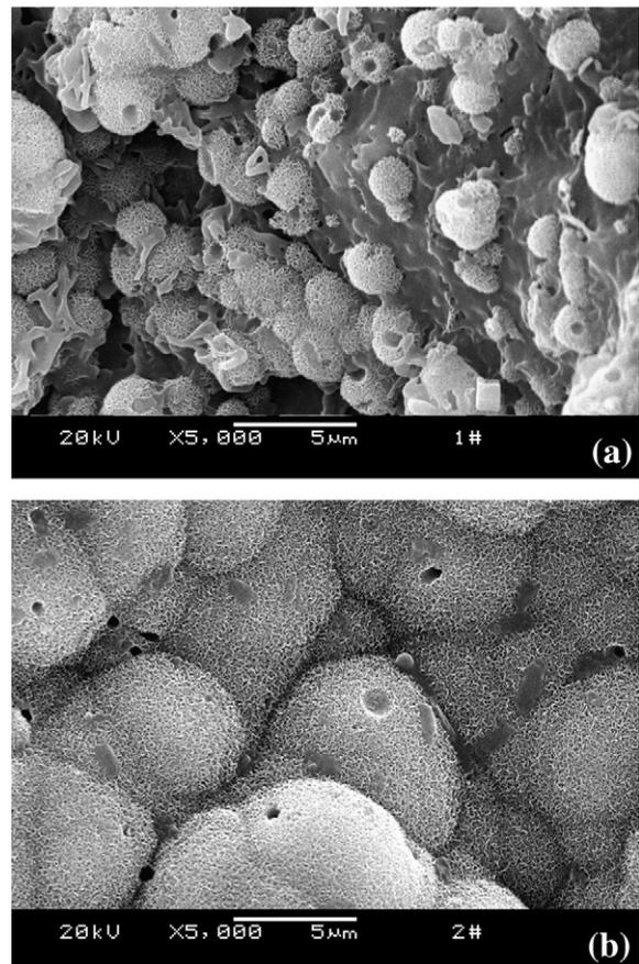
Fig. 3. SEM images of spherical crystals formed on scaffold after 1 week (a) and 2 weeks (b).
