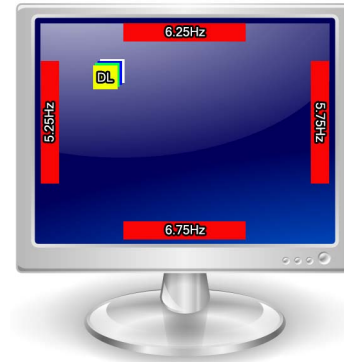
Fig. 3: Screen Stimulus Setup. The red rectangles represent the mouse location stimulus. The Yellow, green, blue, and white squares represent the double left, left, right and no mouse click event stimulus.
